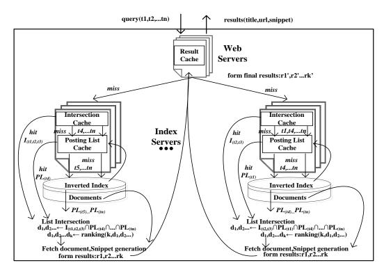
Fig. 2. Caching system architecture in search engine
